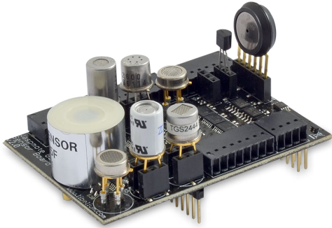
Figure: Gases Board
