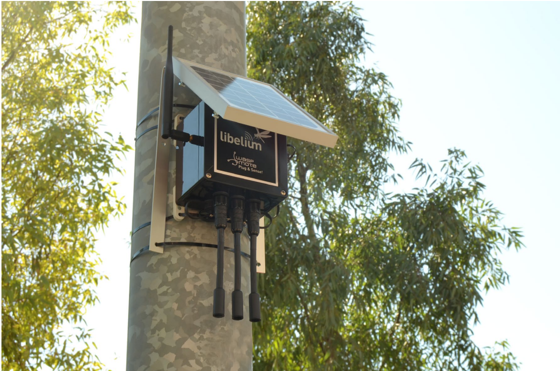
Figure: Wasmote Plug & Sense! powered by an external solar panel
