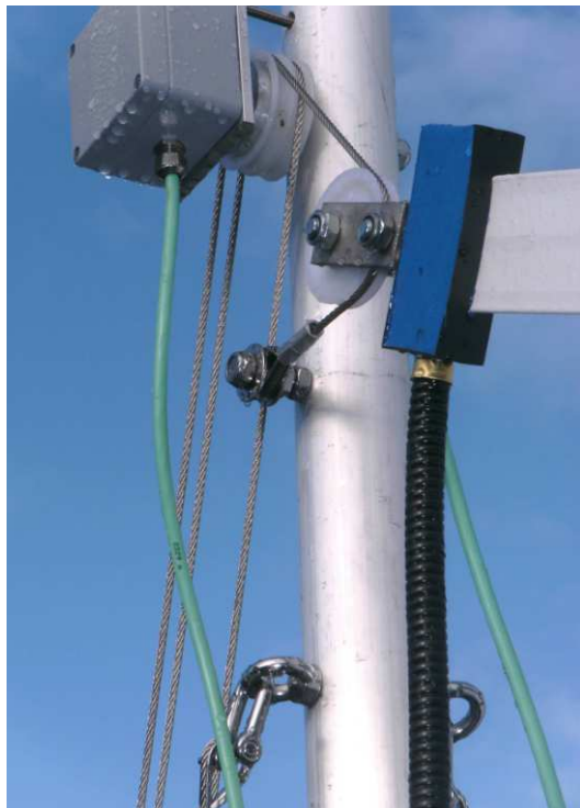
Fig. 9: Upper end of the sloping sensor with the upper part of the tensioner from different views
