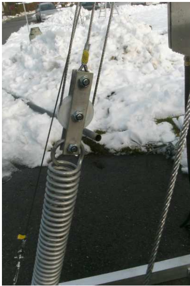
Fig. 10: Suspension at top of the spring with the pulley system (overview and detail)
