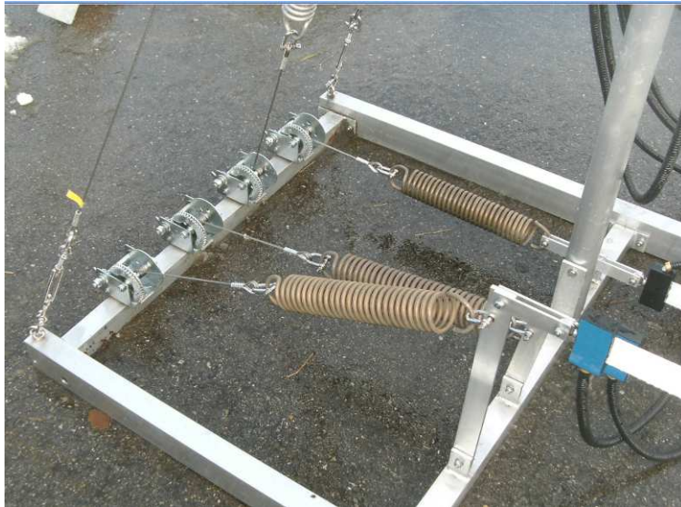
Fig. 11: Spring connection for horizontal sensor
