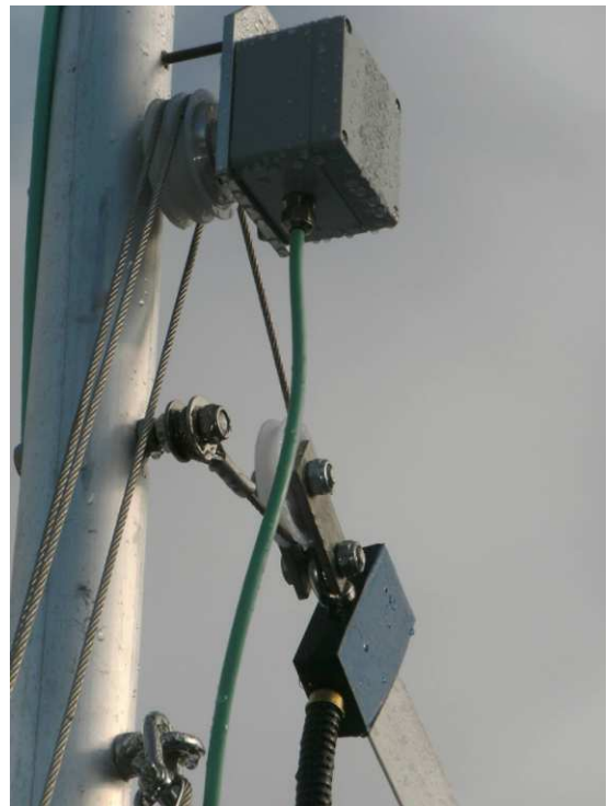
Fig. 9: Upper end of the sloping sensor with the upper part of the tensioner from different views
