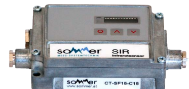
Evaluation electronics in robust zinc die-cast casing
