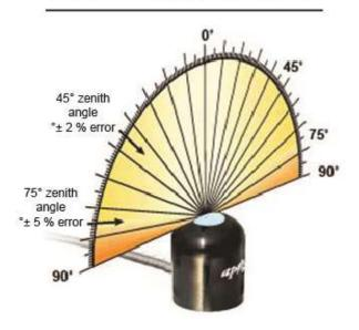
Directional, or cosine, response is defined as the measurement error at a specific angle of radiation incidence. Error for Apogee SQ series quantum sensors is approximately  $\pm 2\%$  and  $\pm 5\%$  at solar zenith angles of 45° and 75°, respectively.
