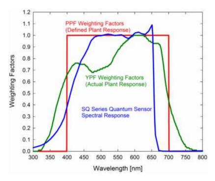
Radiation weighting factors for PPF (defined plant response to radiation), YPF (measured plant response to radiation), and Apogee SQ Series quantum sensors (sensor sensitivity to different wavelengths of radiation).
