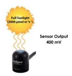
Example of PPF measurement with an Apogee quantum sensor. Full sunlight yields a PPF on a horizontal plane at the Earth's surface of approximately 2000  $\mu mol~m^{-2}~s^{-1}$ . This yields an output signal of 400 mV. The signal is converted to PPF by multiplying by the calibration factor of 5.00  $\mu mol~m^{-2}~s^{-1}$  per mV.
