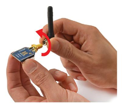
Figure : Plug the antenna to a XBee module
